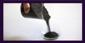
Blacksand Technology was founded to commercialize new titanium production methods developed at the University. Blacksand's process is aimed at making low-cost, high-quality titanium powder for use in emerging methods of manufacturing parts for aerospace and medical implants.
